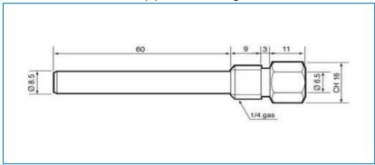
The socket is equipped with a PG7 - IP68 cable gland applied to the hexagonal end to secure the cable. The socket ans sensor need to be installed in accordance with the applicable rules of good workmanship. The socket needs to be installed behind the manifold connecting the coil connections from both sides. The minimum distance between the manifold and the socket is advised to be +- 1 m in order to ensure the flow from both sides is well mixed and the correct temperature is relayed to the PLC.
