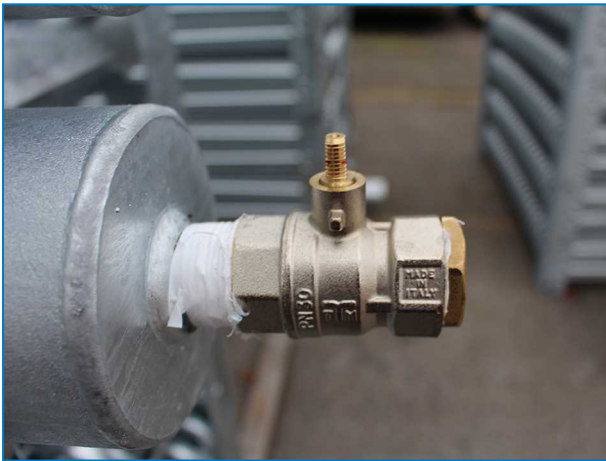
Non-threaded coil connection with pressure release valve on ice thermal storage unit for direct refrigerant feed.
