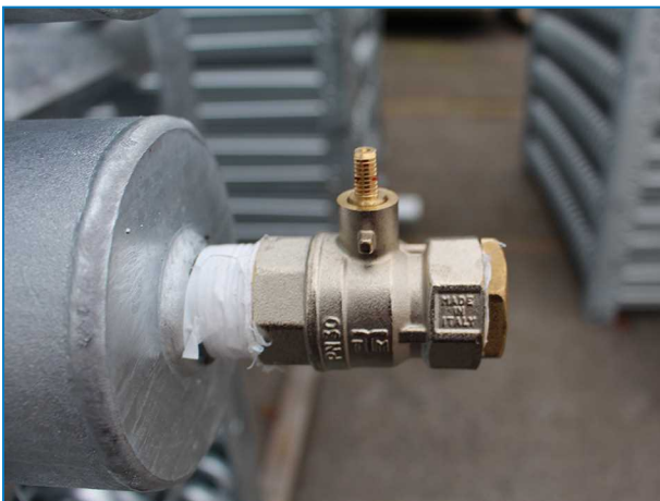
Non-threaded coil connection with pressure release valve on ice thermal storage unit for direct refrigerant feed.
