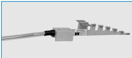
A series of accurately positioned electrodes detect the ice thickness on the coil tube. The measurement is based on the difference in electrical conductivity between ice and water. The Ice Logic™ ice quantity controller combined with this sensor permits to limit the maximum ice thickness to typically 35 mm.
