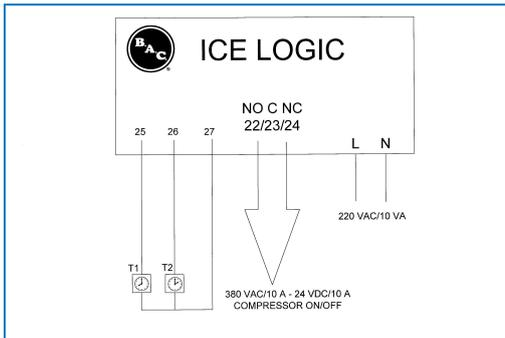
The required ice quantity for the next cooling cycle can easily be set from the control panel in steps of 20%. In addition, the minimum ice quantity, before the cooling equipment should start again, can be set from the minimum % ice knob. If a minimum of 0% is selected, the compressor will not be allowed to start before all ice is melted. Use contact 22/23 NO or 23/24 NC to start or stop the compressor as a function of predetermined minimum and maximum ice quantity.
