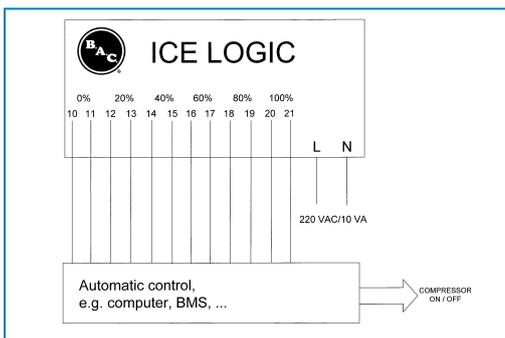
The Ice Logic™ ice quantity controller has six output contacts (NO) which can be used to control the cooling equipment. These contacts are normally open and will close when the desired ice quantity is reached.
