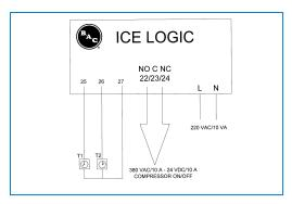
The required ice quantity for the next cooling cycle can easily be set from the control panel in steps of 20%. In addition, the minimum ice quantity, before the cooling equipment should start again, can be set from the minimum % ice knob. If a minimum of 0% is selected, the compressor will not be allowed to start before all ice is melted. Use contact 22/23 NO or 23/24 NC to start or stop the compressor as a function of predetermined minimum and maximum ice quantity.
