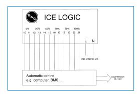
The Ice Logic<sup>™</sup> ice quantity controller has six output contacts (NO) which can be used to control the cooling equipment. These contacts are normally open and will close when the desired ice quantity is reached.
