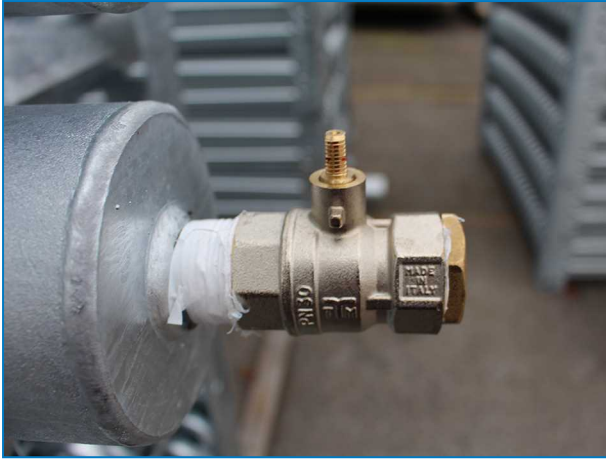
Upper coil connection with pressure release valve on condensers.
