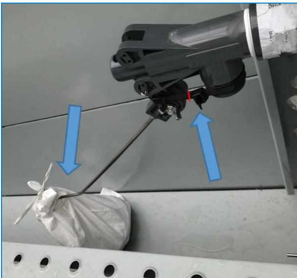
Fixation and wrapping of float ball
