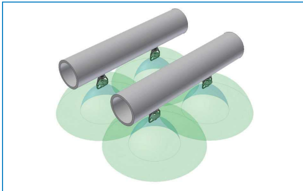
Nozzle spray distribution type for condenser
