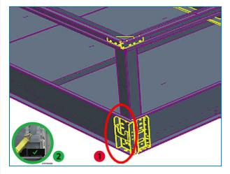
Position tie-down buckle on water collection module
