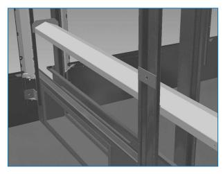
Water baffle Installation – Step 1
