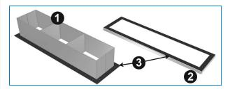
Sealing method for installation of flume box
