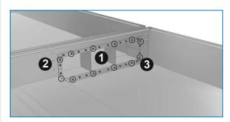
Remove indicated tappers/bolts befor installation of positive closure plate.
