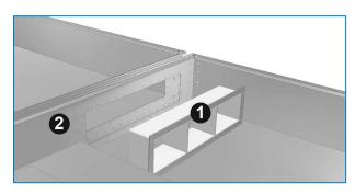
Sliding of flume box into whole between Cell#1 and Cell #2
