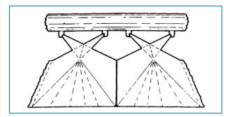
Nozzle spray distribution type cooling tower
